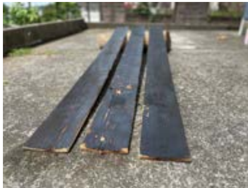
Fig32. Photos in the process of "Yakisugi" 20
